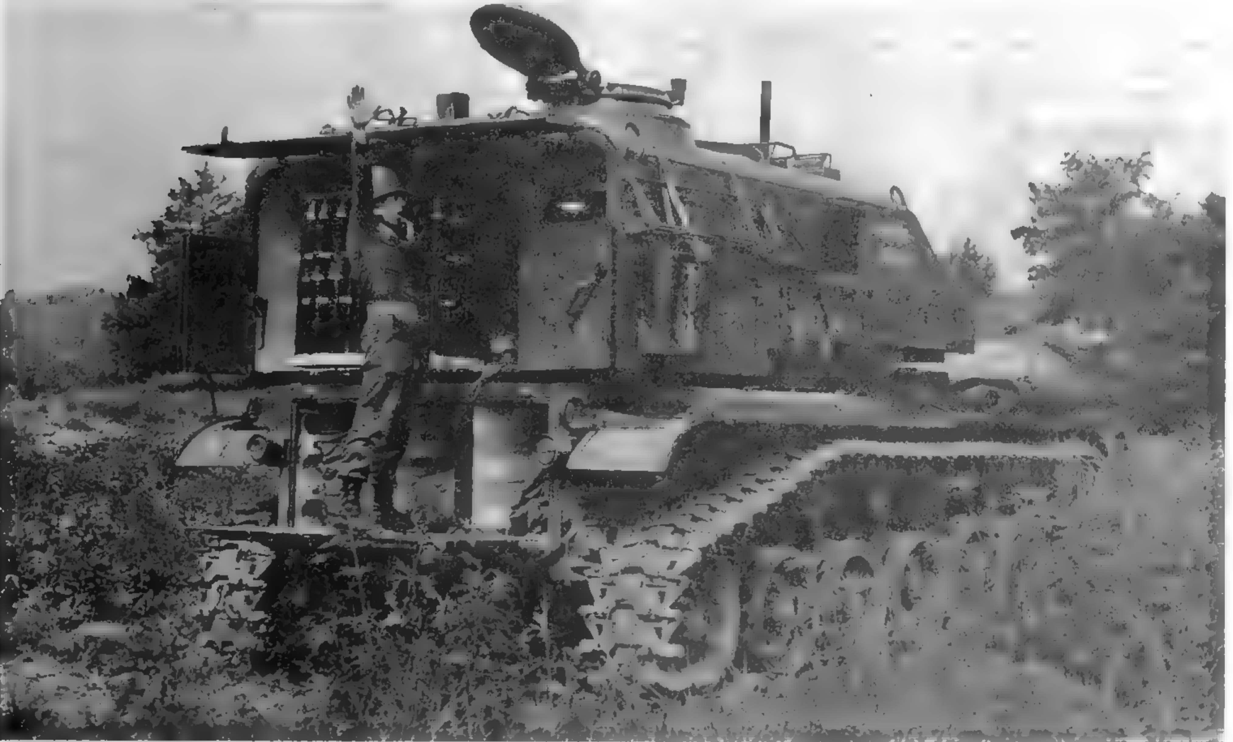
This M52 has moved into position and is preparing to fire. The rear of the armored turret opened and a deck for the gun crew swung down from the hull. (Photo courtesy of the Patton Museum)
